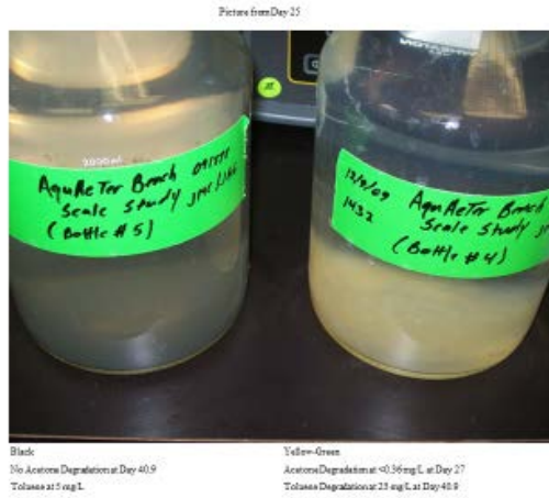
Figure 11. Bottle bacterial populations require about 2 weeks to establish an acclimated population for the source organics, as well as most biological systems
