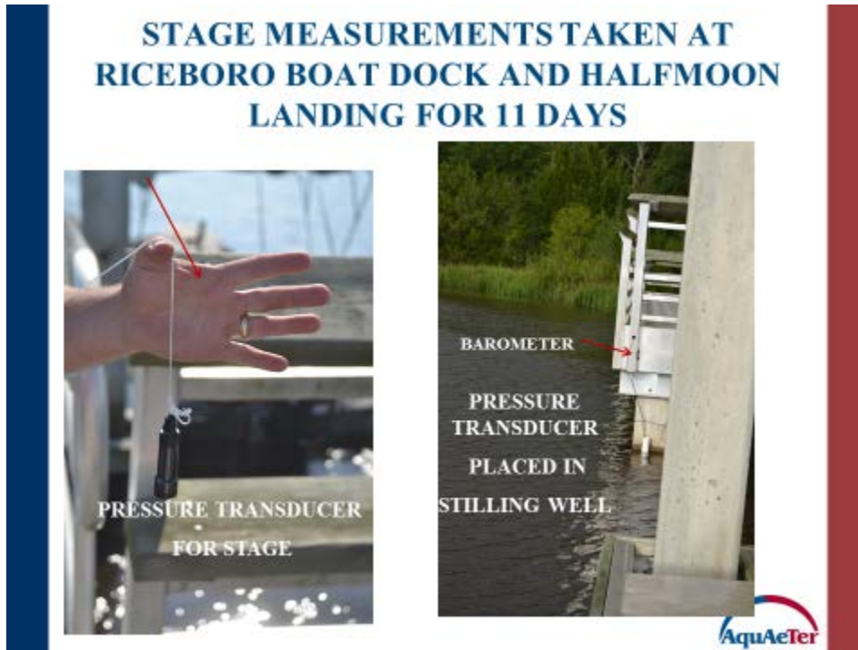
Figure 26. Stage and barometric pressure recordings can be done economically
